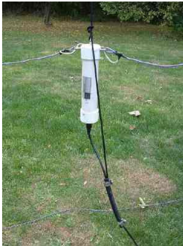
Inverted Vee Center Details
